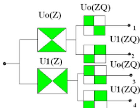
Figure 2: Four-channel non-subsampled directional filter bank.
