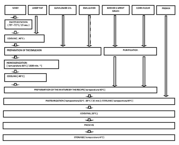
igure - 1 Technological scheme for the preparation of liquid milk replacer for calves
