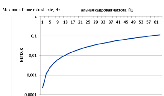
Fig. 5. Relationship between NETD and maximum frame refresh rate with consideration of optimization of doping of a polycrystalline silicon of the thermocouple (membrane \text{SiO}_2 , t_m = 0.2 \mu\text{m} , t_r = 0.2 \mu\text{m} , l_r/w_r = 25 , N_r = 1 , \chi_r = 30 \text{ V/m} \cdot \text{K} , c_m = 1.9 \cdot 10^6 \text{ J/m}^3 \cdot \text{K} , \rho_r = 12 \Omega/\text{sq} , \alpha_r = 84 \mu\text{V/K} , matrix 64 \times 64 )
