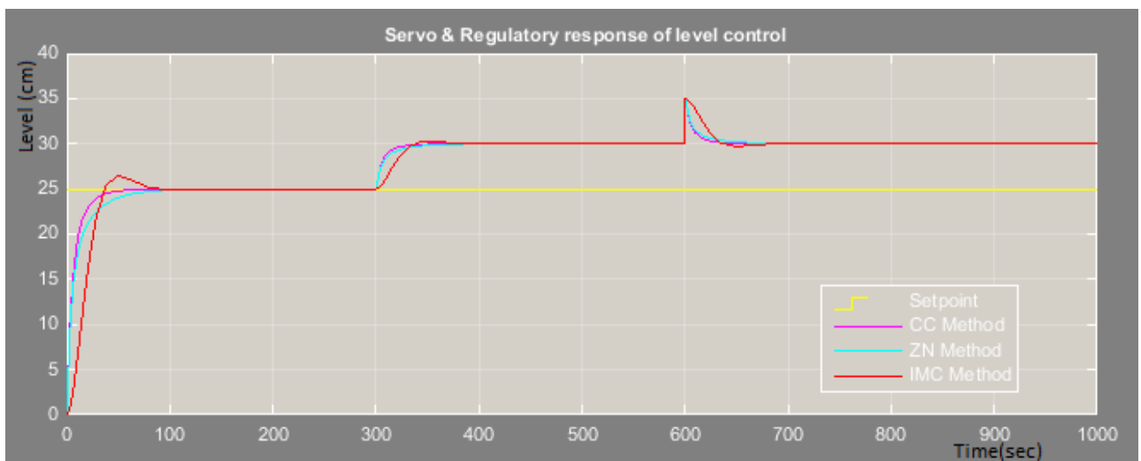
Figure 7: Level control for the process for a setpoint of 25 cm having the setpoint tracking and Load disturbances
