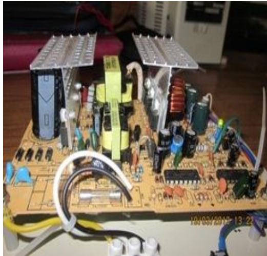
Figure 13: Experimental Set Up of Step-down converter in Side View
