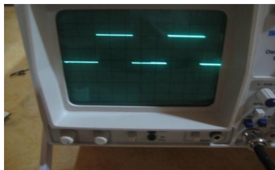
Figure 16: Oscillogram of Driving pulses
