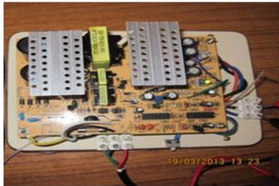
Figure 14: Experimental Set Up of Step-down converter in Top View
