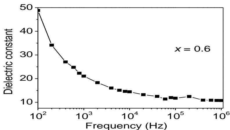
**Figure 4: Frequency dependence of dielectric constant of  $\text{Sr}_{1-x}\text{Bi}_{3+x}\text{LaTi}_{4-x}\text{Mn}_x\text{O}_{15}$  with  $x = 0.6$  synthesized by hydrothermal technique.**
