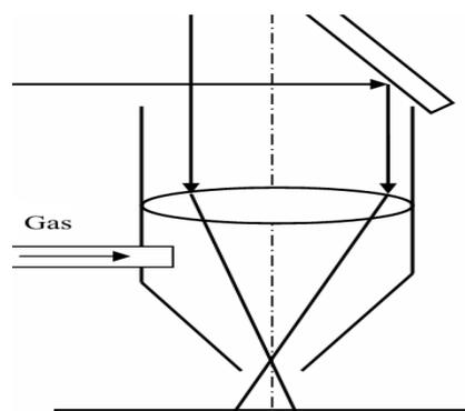
**Fig.2. Diagram of the process of the formation of pores on the surface of an implant**
