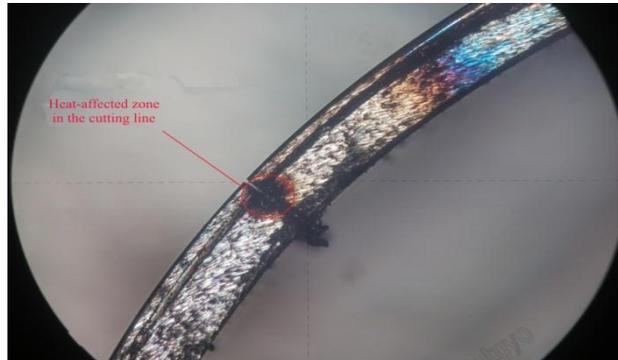
**Fig.2. Heat affected zone inside the cut line at a slight increase of the radiation frequency**
