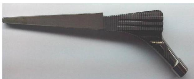
**Fig.4. General view of the sample of the femoral component of the hip prosthesis with developed surface**
