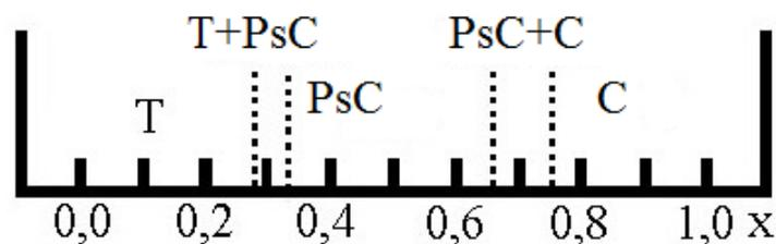
Fig. 1. Phase state diagram of the  $Ba_{1-x}Sr_xTiO_3$  system.
