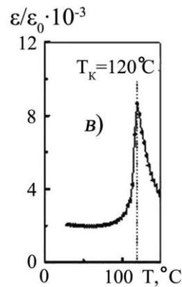
**Fig. 6. Relationships of relative dielectric permeability,  $\epsilon/\epsilon_0$ , and temperature of  $\text{BaTiO}_3$  a) – [3]; b) – [1]; c) – the obtained data.**
