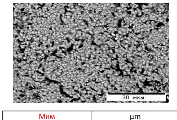
**Fig. 2. Fragments of microstructure of ceramics of SS of the system  $(1-x) \text{BaTiO}_3-x\text{SrTiO}_3$  in the interval  $0.0 \leq x \leq 1.0$  (Figure shows values of  $x$ ).**
