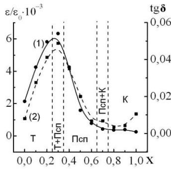
Fig. 5. Relationships of relative dielectric permeability,  $\epsilon/\epsilon_0$ (1), dielectric dissipation factor  $\text{tg} \delta$  (2) TP (1-x) BaTiO<sub>3</sub>-xSrTiO<sub>3</sub> and concentration of SrTiO<sub>3</sub>.
