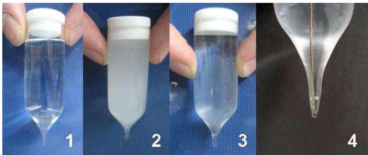
**Figure 3: Scheme of microextraction concentration with dispersion of the extractant (1 - initial aqueous condensate analyze, 2 - emulsion in water after the addition of the extractant with a dispersing agent, 3 - extract isolated after centrifugation, 4 – sampling of extract).**
