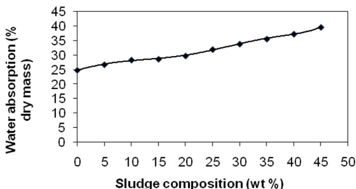
Figure 1: Effect of sludge composition on the water absorption of bricks
