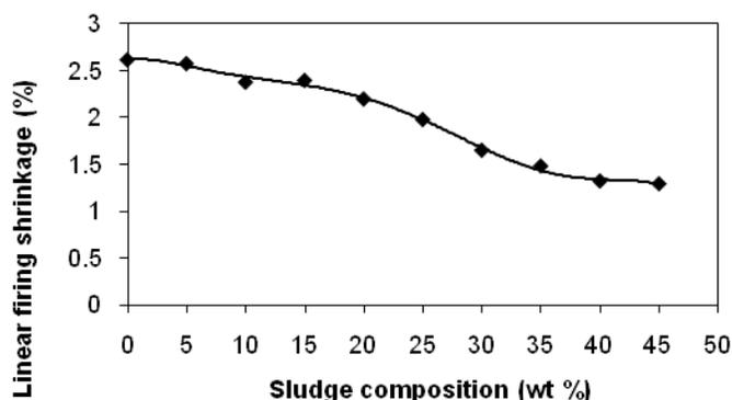
Figure 2: Effect of sludge composition on linear firing shrinkage
