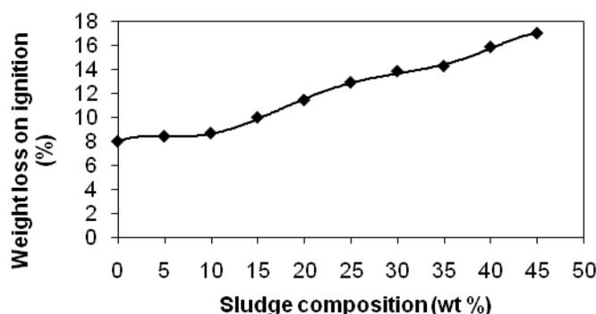
Figure 3: Effect of sludge composition on weight loss on ignition after firing
