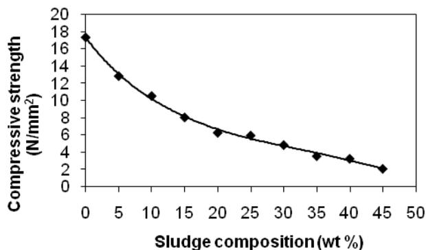
Figure 4: Effect of sludge composition on compressive strength
