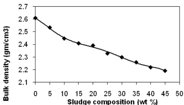
Figure 5: Effect of sludge composition on bulk density
