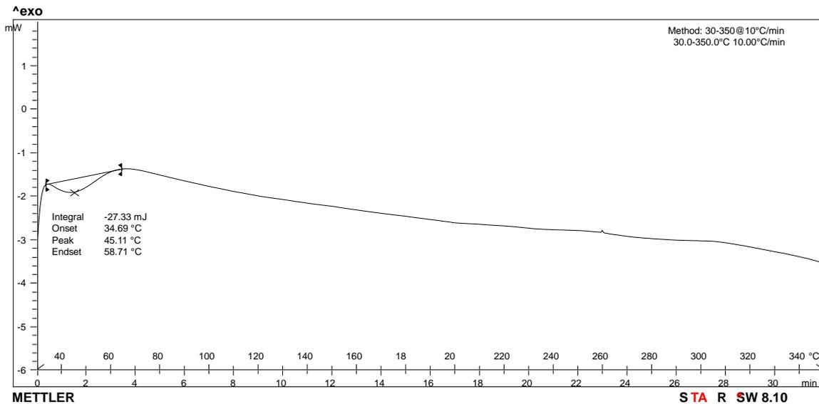
Figure 2: DSC curve of HPC-SL (carrier)
