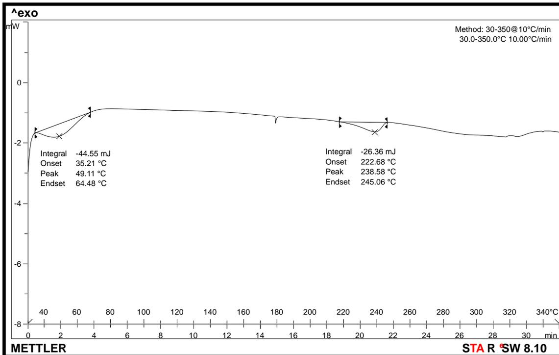
Figure 4: DSC curve of drug, polymer and vitamin-E.TPGS
