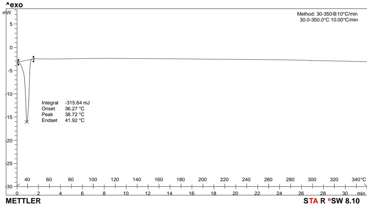
Figure 3: DSC curve of vitamin-E.TPGS (Plasticizer)
