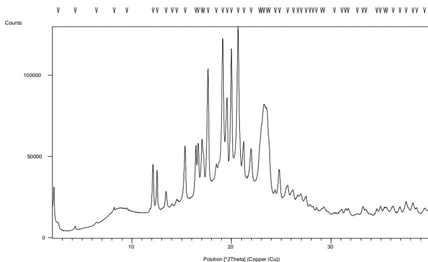
**Figure 6: PXRD of Solid dispersion**
