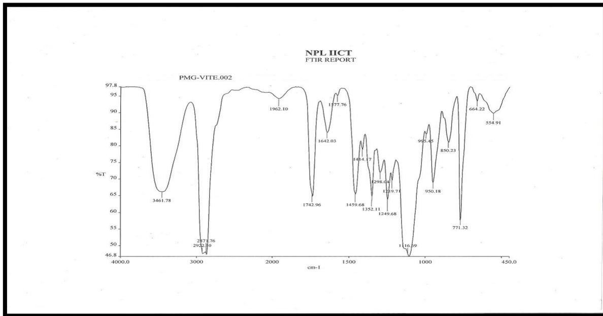
Figure 8: FTIR spectra of vitamin-E, TPGS
