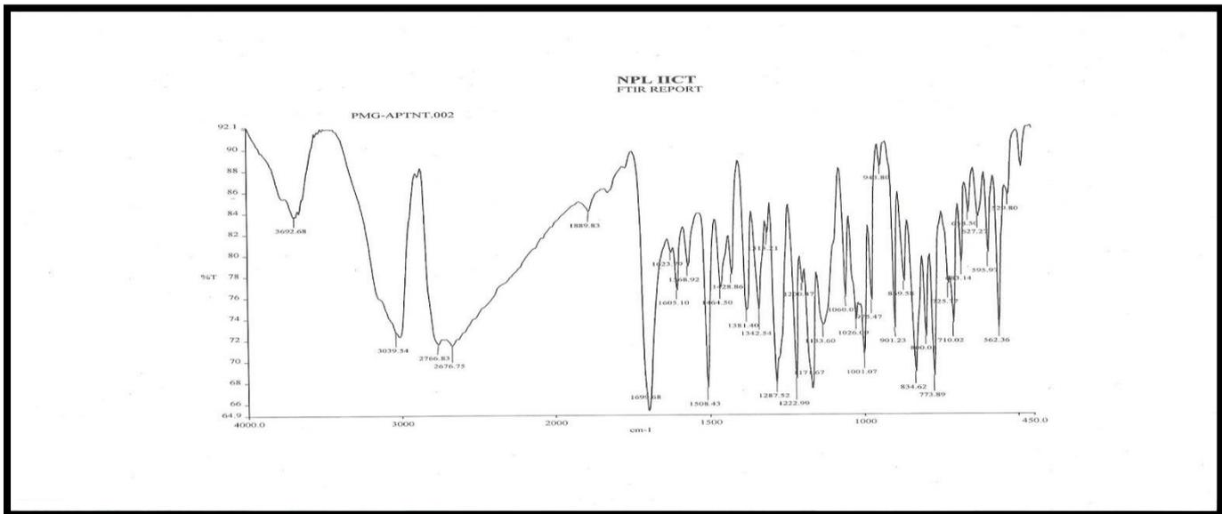
Figure 10: FTIR spectra of Solid Dispersion formulation of aprepitant
