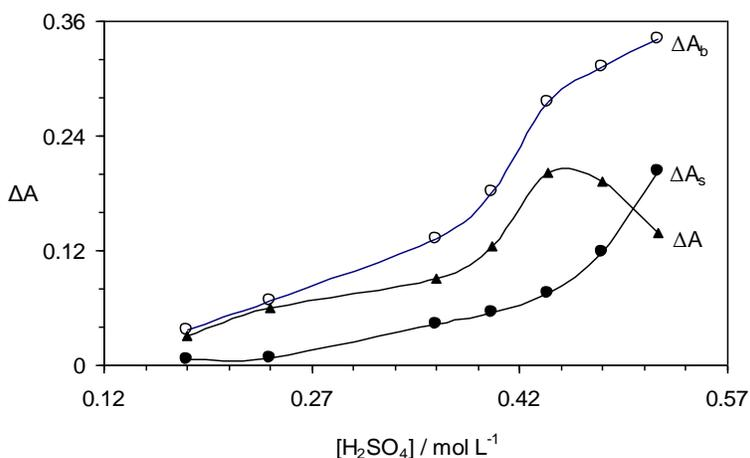
**Fig. 3:** Effect of sulfuric acid concentration on the rate of uninhibited ( $\Delta A_b$ ), inhibited ( $\Delta A_s$ ) reactions and response ( $\Delta A$ ). (Conditions: Orange G,  $66.0 \mu\text{mol L}^{-1}$ ; codeine,  $25.0 \mu\text{mol L}^{-1}$ ; bromate,  $2.5 \text{ mmol L}^{-1}$ ;  $25^\circ\text{C}$  and 450 s).
