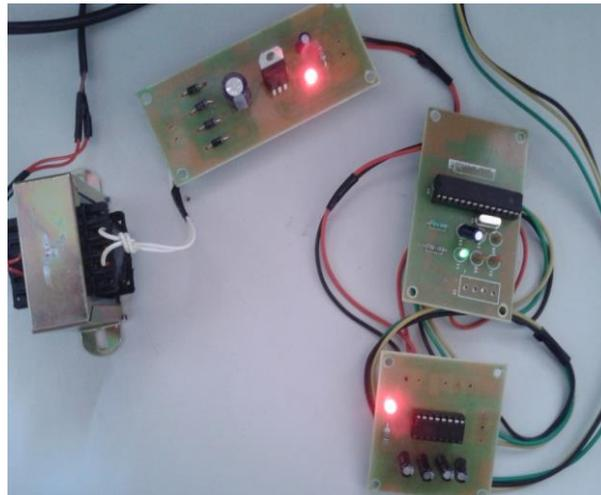
Figure 12: ZigBee Transmitter
