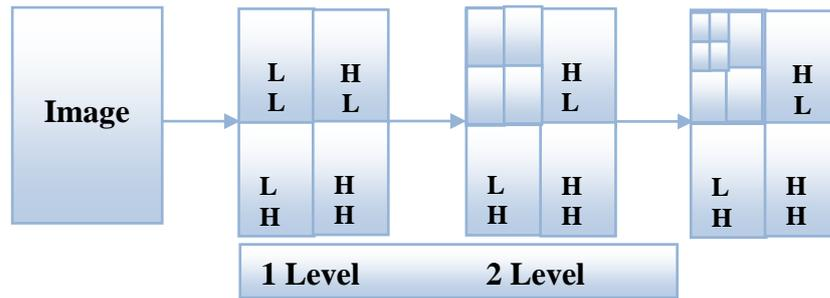
Figure 2: Discrete wavelet transforms (2D-DWT) operation
