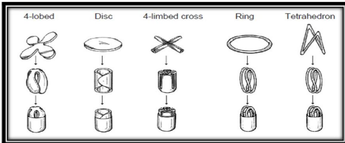
Fig. 6: Different geometric forms of unfoldable systems [15]
