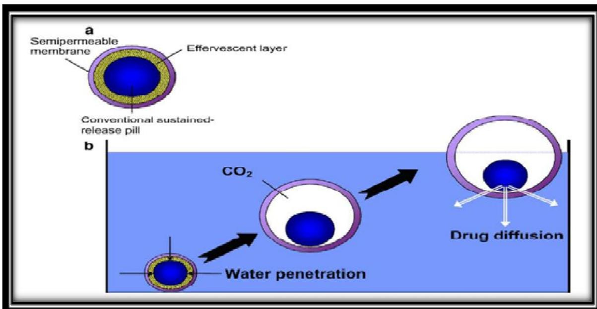
Fig. 3: Schematic representation of "floating pill" proposed by Ichikawa (a). The penetration of water into effervescent layer leads to a CO<sub>2</sub> generation and makes the system float (b). Adapted from Ichikawa et al. Used with permission. [15]
