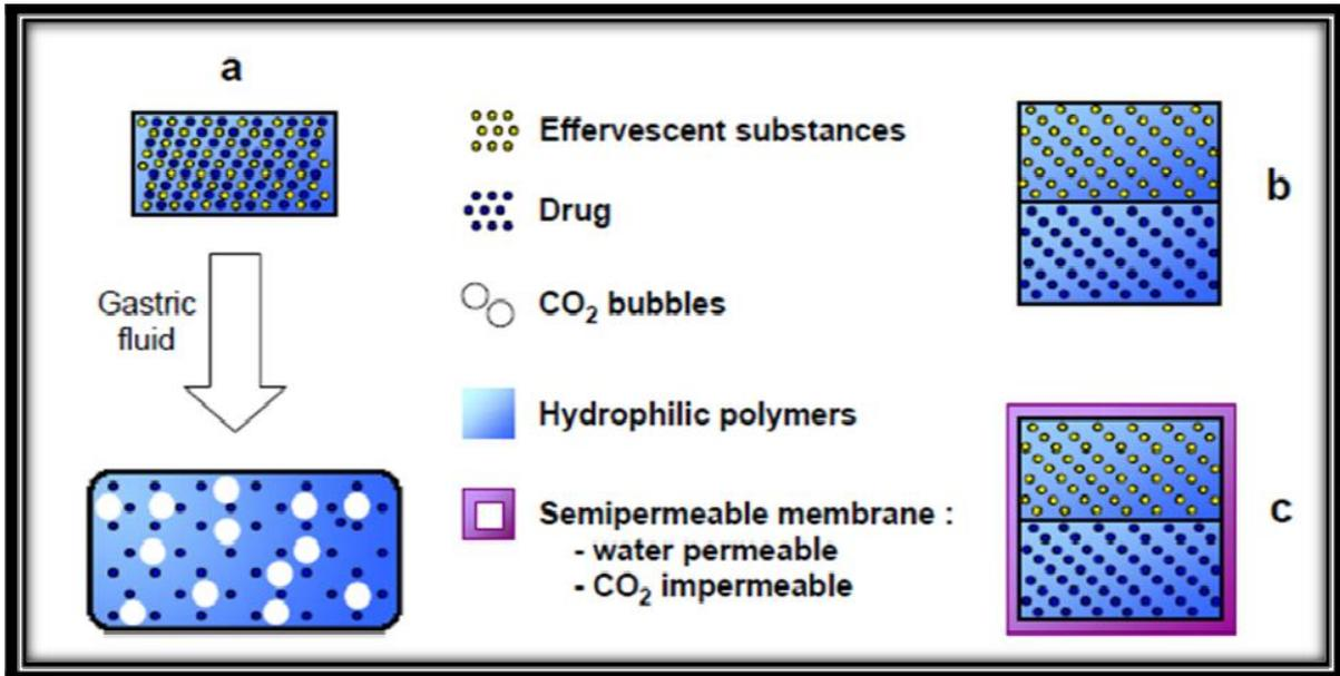
Fig. 2: Gas-generating systems. Schematic monolayer drug delivery system (a). Bilayer gas-generating systems, with (c) or without (b)
