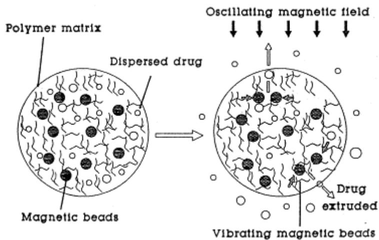
Fig.10: Mechanism of magnetic system.
