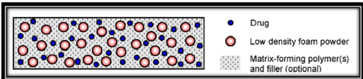
Fig. 4: Schematic presentation of the structure of the low-density, floating matrix tablets. Adapted from Streubel et al. Used with permission. [15]
