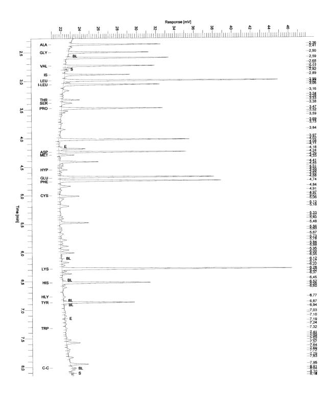
Fig. 4. Chromatogram sample of Aminogame 1500 solution, hydrolysed with 6M HCl for 72 h at 110°C.
