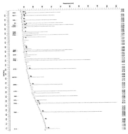
Fig. 1. Chromatogram of reference standard solution of aminoacids, used for the calibration before the analysis of free aminoacids in sample of Aminogame 1500 solution.
