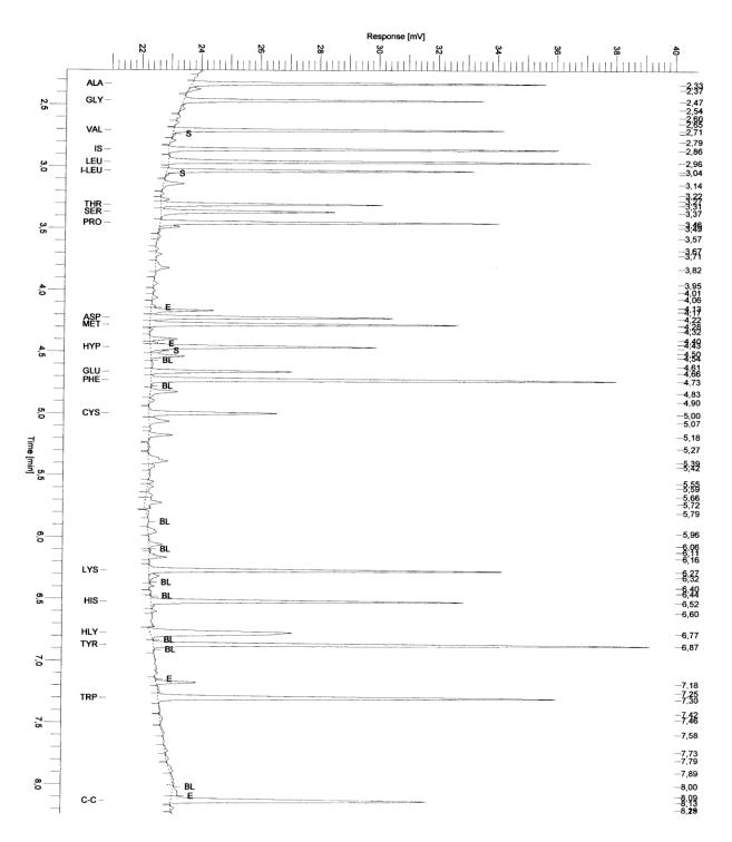
Fig. 3. Chromatogram of reference standard solution of aminoacids, used for the calibration before the analysis of acid hydrolysed sample of Aminogame 1500 solution.
