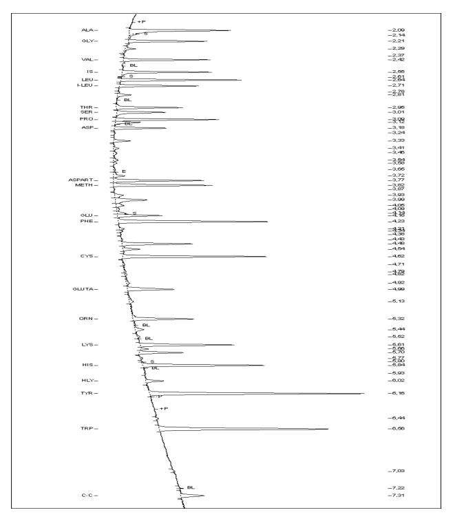
Fig. 5. Chromatogram of reference standard solution of aminoacids, used for the calibration before the analysis of alkaline hydrolysed sample of Aminogame 1500 solution
