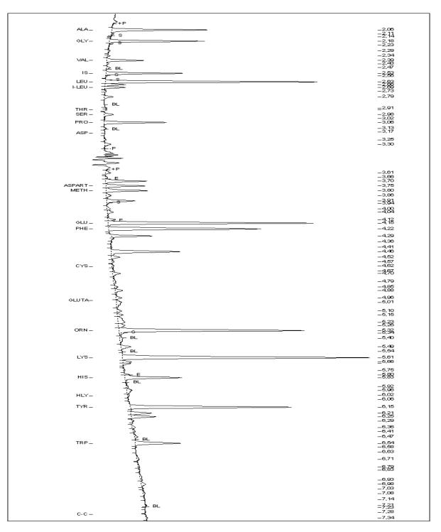
Fig. 6. Chromatogram of sample of Aminogame 1500 solution, hydrolysed with 1M KOH for 48 h at 110°C
