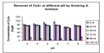
Fig.1 Removal of Cu (II) at different pH by growing A.lentulus
