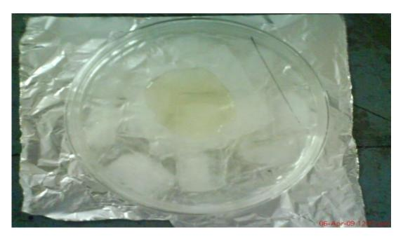
Fig.1. Gelatin membrane casting on nylon piece (transparent) under low temperature condition.
