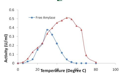
Fig 2: Effect of temperature on the activity of soluble and immobilized amylase.
