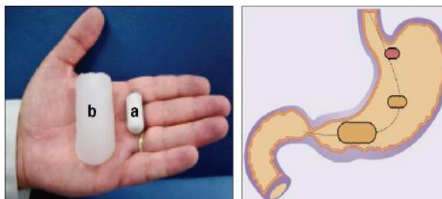
Figure 7: On the left, Superporous Hydrogels in its dry (a) and water-swollen state (b) On the right, schematic illustration of the transit of Superporous Hydrogels.
