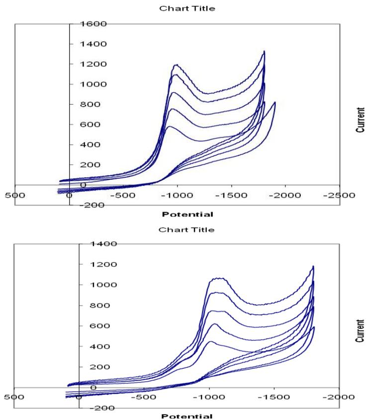
Fig.2. Cyclic voltammograms of Benzylidene acetone at pH 5.0, 7.0 & 9.0 (At variable scan rates from 100 to 500 mV/sec)
