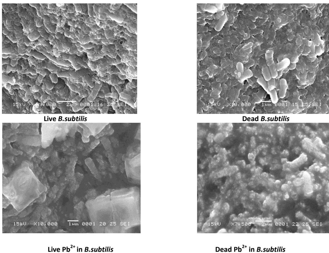
Fig. 6. Scanning electron micrograph of live and dead *Bacillus subtilis* and  $Pb^{2+}$  ions.
