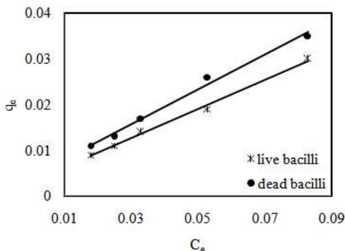
**Fig. 2.** Langmuir isotherms of  $Pb^{2+}$  ion on live and dead biomass of *B.subtilis*.
