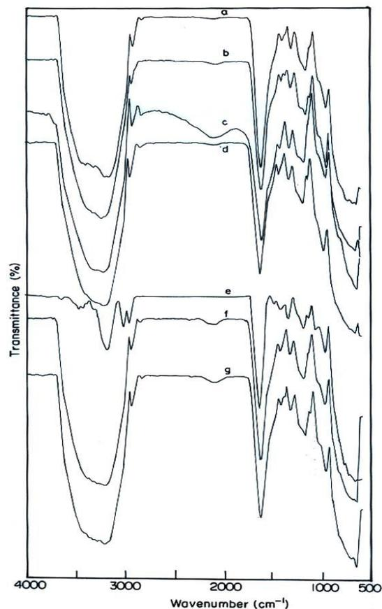
**Fig. 5. Infra spectra of (a) live *B.subtilis* were treated with Pb<sup>2+</sup> ions for different lengths of time namely (b) 0.0, (c) 0.2, (d) 0.12, (e) 0.24 hrs, (f) dead *B.subtilis* and (g) dead Pb<sup>2+</sup> ion.**
