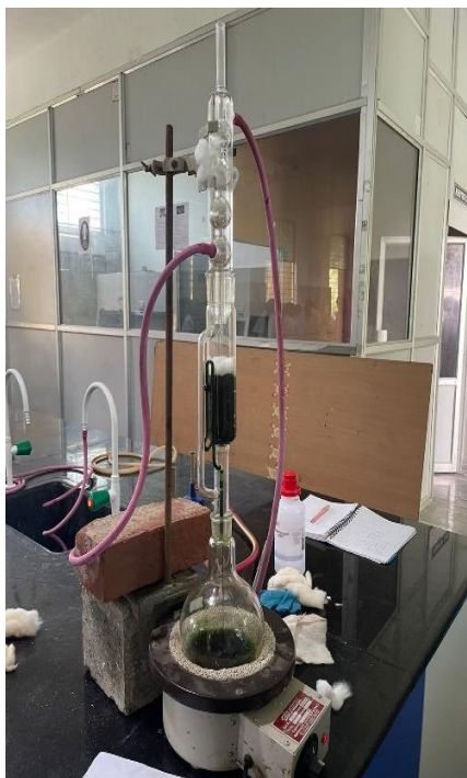
Figure 2: Extraction of Tridax procumbens using Soxhlet Apparatus
