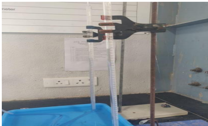
Figure 5: Inverted Burette for Biogas production measurement.
