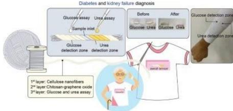
Figure 7. Abstract procedure of the fabricated cotton thread-based biosensor. [16]
