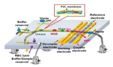
Figure.1. Schematic of the enzyme-doped thread coated with PVC membrane for highperformance CE-EC detection.[9]
