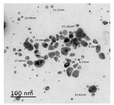
Fig. 4 TEM micrograph of the biosynthesized AgNPs
