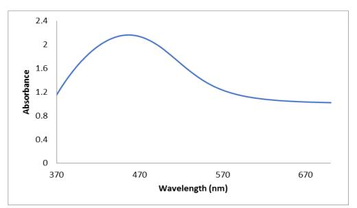
Fig. 3 UV-Vis spectra analysis of the produced AgNPs in the presence of sunlight after 111 days.
