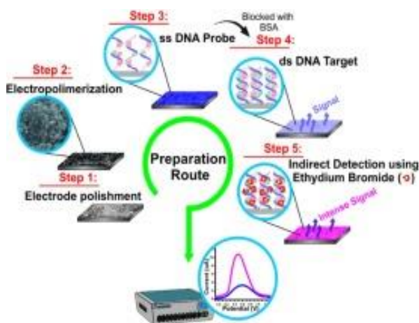
Fig 9: The following steps are engaged for detection method- electrode modification, hybridization, washing and electrochemical transducer [43]
