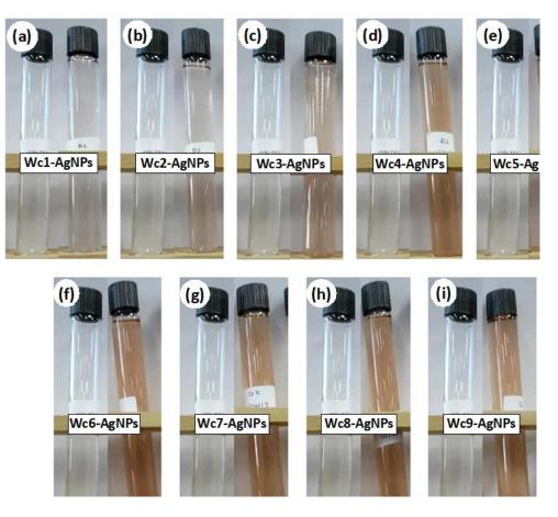
Fig.1: Visual observation for colour changes of silver nanoparticles for all samples : (a) Wc1-AgNPs, (b) Wc2-AgNPs, (c) Wc3-AgNPs, (d) Wc4-AgNPs, (e) Wc5-AgNPs, (f) Wc6-AgNPs, (g) Wc7-AgNPs, (h)Wc8-AgNPs, (i) Wc9-AgNPs after 8 minutes incubation reaction.
