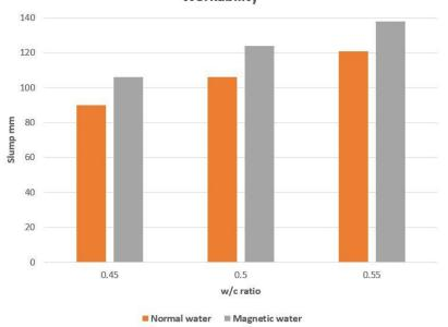
Figure 3 Variation of slump with w/c ratio
