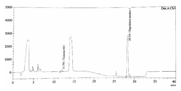
Figure 5. Oxidative degradation chromatogram of TNT
