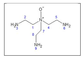
Figure 12. Proposed structure of TNT Degradation product
