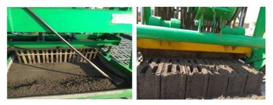
Figure 1: Preparation of slag concrete hollow blocks
