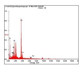
Figure 5: Energy Dispersive X-Ray Analysis image of slag concrete
