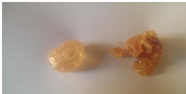
Fig 1: Two Gum Arabic varieties of Acacia types, A. Senegal: almost colorless ( to your left hand); A. seyal: brown to reddish color (to your right hand).
