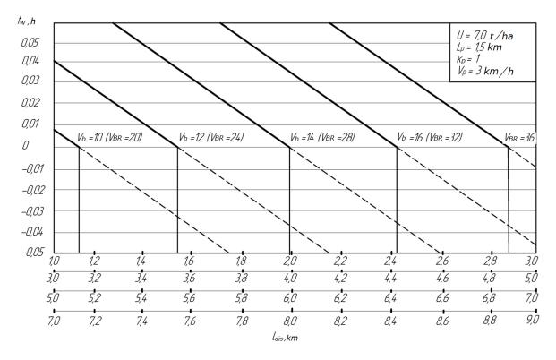
Figure 4: The dependence of the criterion for optimizing  $t_w$  on the capacity of the drive - reloader and distances  $I_{dis}$  at a yield of 7 t / ha
