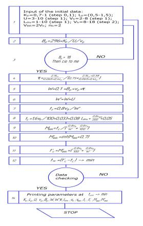
Figure 2: The block diagram of the optimization of the work of the harvest-transport link (HTU)
