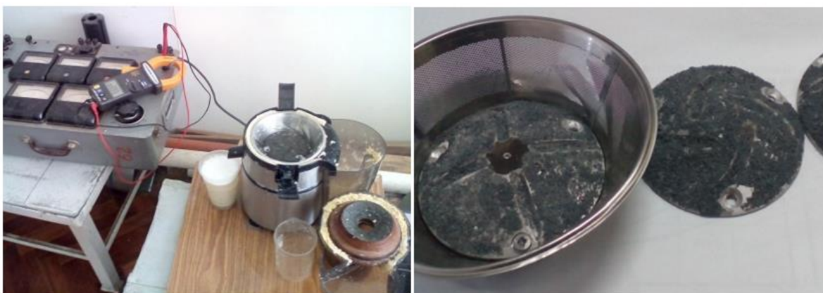
Figure 4: General view of the grain grinder in a soaked form with interchangeable abrasive discs
