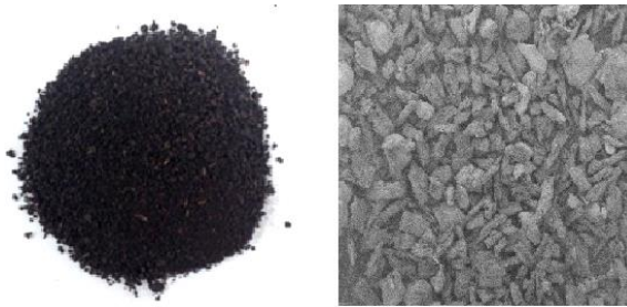
Figure 1: Solid product of processing of sludge of sewer sewage
