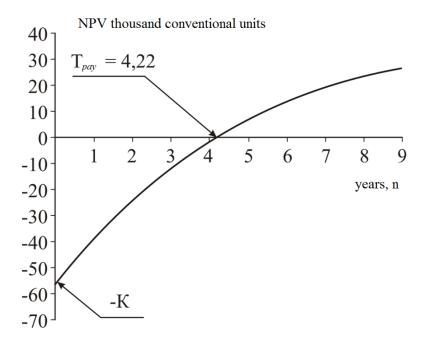
Figure 1: Graphic determination of dynamic payback period
