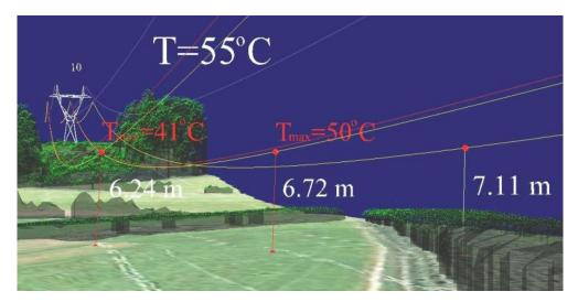
Figure 2: 3D model of power line
