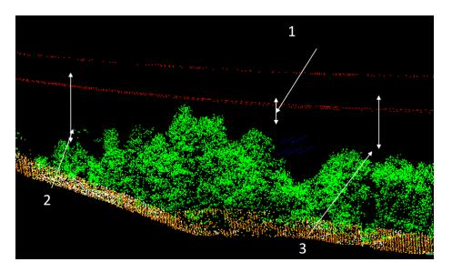
Figure 1: Based on the results of laser scanning, we determine: 1 - distance to the intersected line; 2 - distance to the ground; 3 - distance to vegetation
