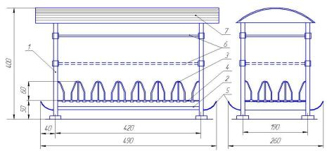
1 - stand; 2 - bottom; 3 - dividing grid; 4 - bar; 5 - feed catchers; 6 - limiter; 7 - roof
