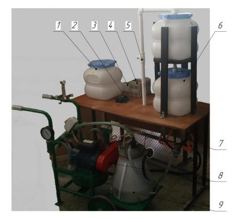
Figure 2: General view of the laboratory stand for research of a milking machine with stepped nipple tubes:
