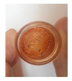
Figure 2: Lycopene crystals after the recrystallization process
