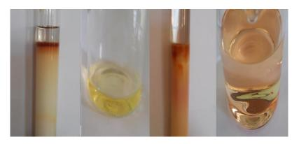
Figure 3: Separation of  $\beta$ -caroten (yellow fraction) and lycopene (red-orange fraction) by column chromatography
