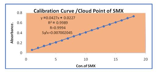
Figure 2-5: Calibration Curve AZO + Cloud Point of SMX
