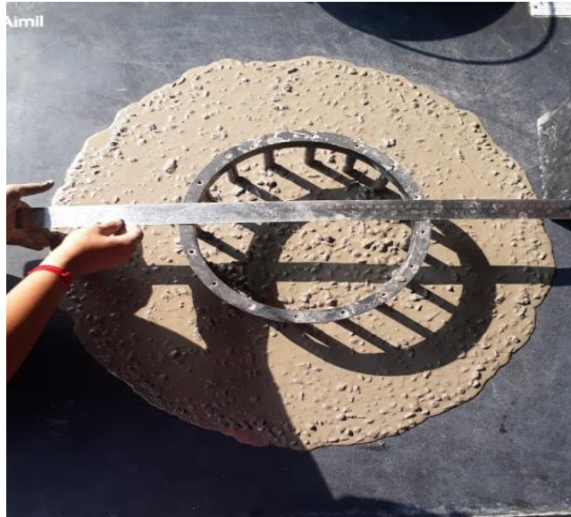
Figure 3 J-ring pasty phase test
