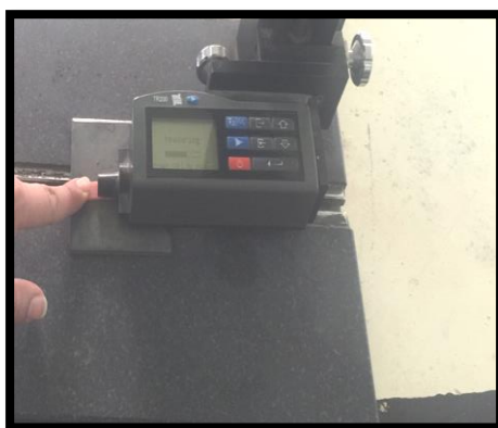
Figure 4: The profilometer device
