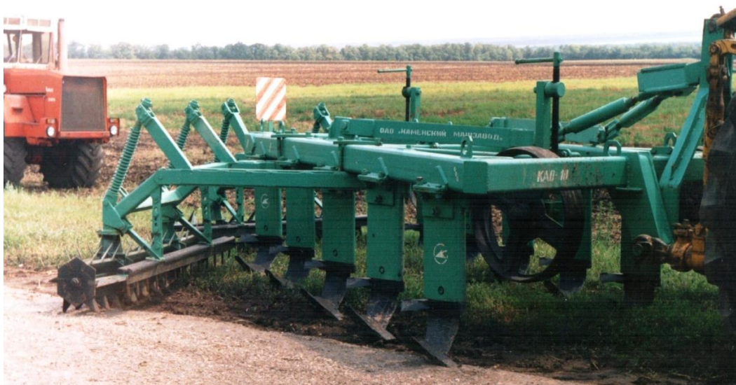
Figure 3: Combined tools with new working elements for traction power facilities 3 and 5
