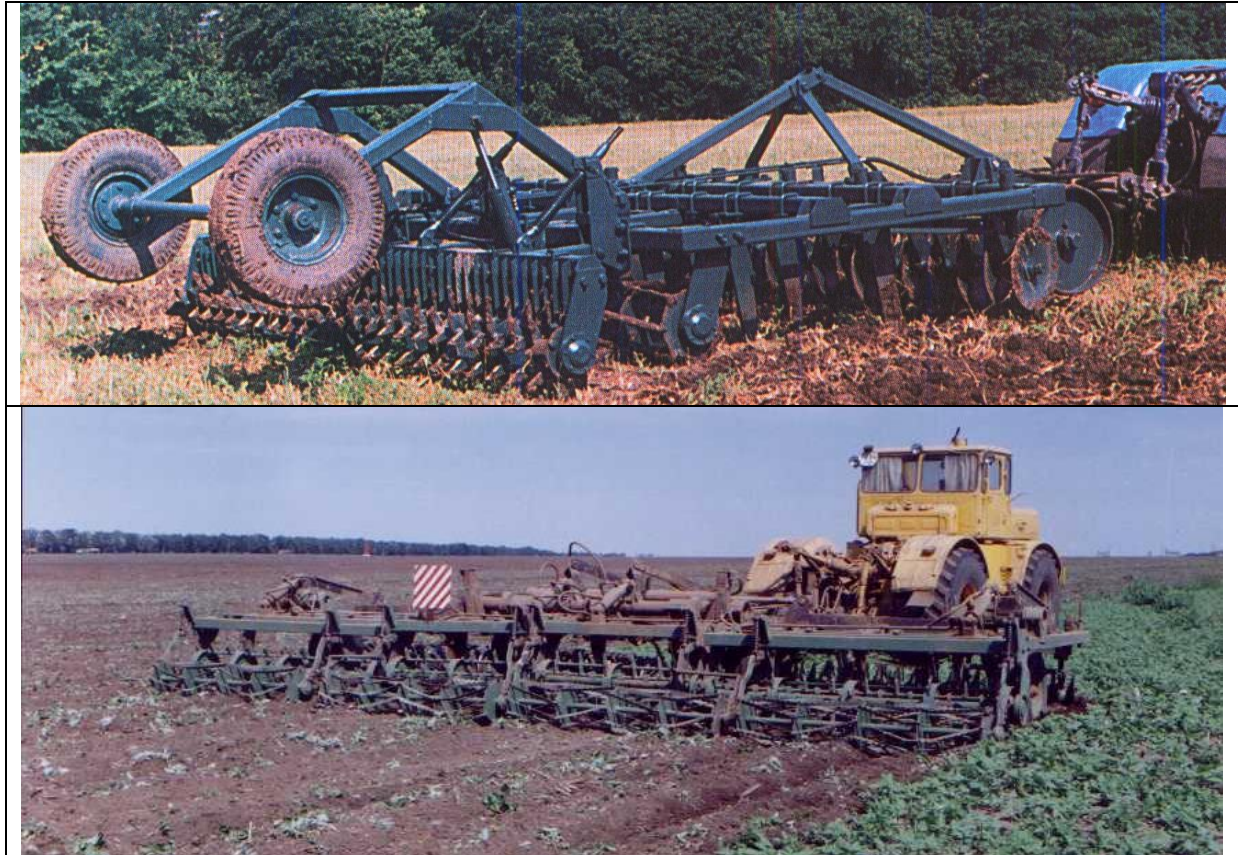
Figure 7: Combined units made according to the proposed schemes for tractors of traction class 3 and 5
