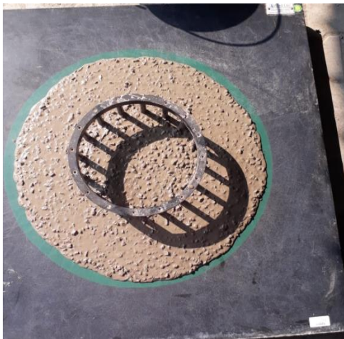
Figure 3: J-ring Test pasty phase test;
