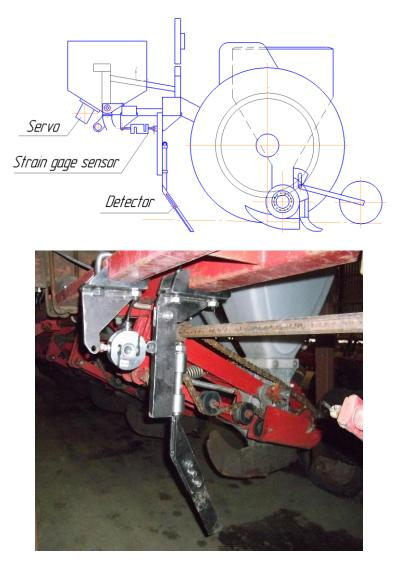
Figure 5: The scheme of installation of devices on a sowing machine
