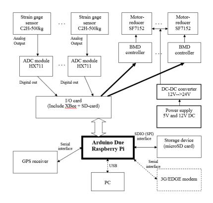
Figure 7: The generalized block scheme of the system for differentiated fertilizer application
