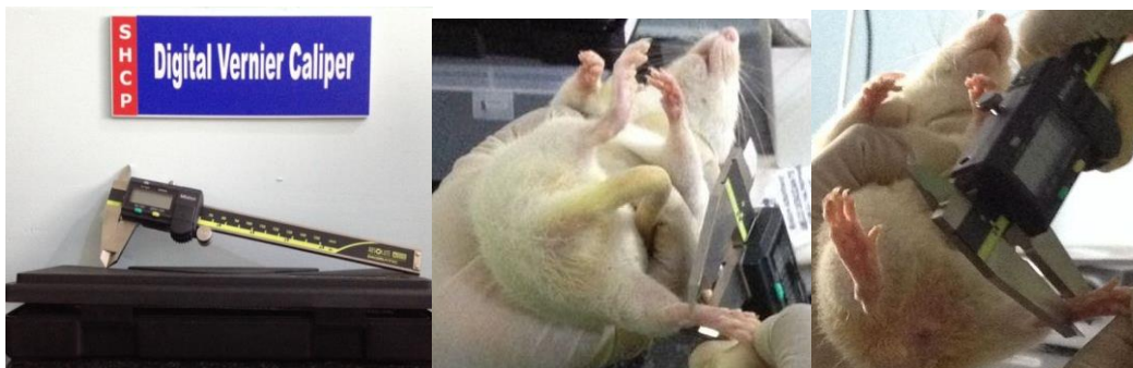
Figure 5: Digital Vernier Caliper Figure 6 & 7: Recording of Paw diameter using digital vernier calipers
