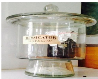
Figure 4: Marc of crude drug set for drying in Desiccator
