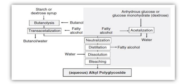
Figure 2: Manufacturing process for alkyl polyglycosides [25]
