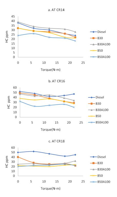
Figure 4: Variation of Hydrocarbon emissions with torque at different Compression ratios
