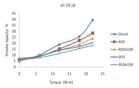
Figure 6: Variation of Smoke Opacity with torque
