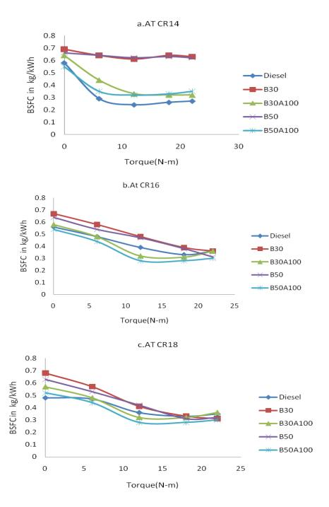
Figure 2: Variation of Brake specific fuel consumption with torque at different compression ratios
