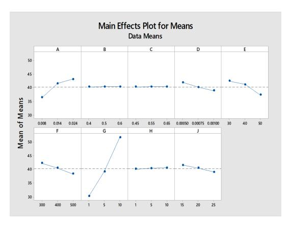
Fig 8: Mean effect of parameters to Air outlet temperature
