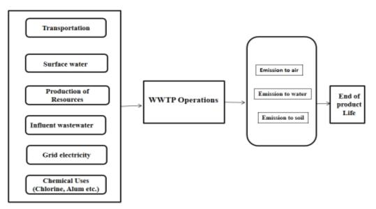
Fig 1: Scope and system boundary of investigated lifecycle
